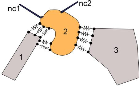
Figure 5: A contact island composed of two individual contact objects, i.e., the tools (*nc1*) and (*nc2*), and one coupling island, formed by contact objects (1), (2) and (3).
